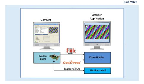
The Gidel **CamSim™** is a flexible high-performance camera simulator that generates CoaXPress and camera link video stream and test patterns for testing frame grabbers or vision/imaging systems. The system supports all CoaXPress and Camera Link™ v2.0 configurations.
