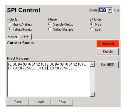
Figure 17 : SPI Slave tab in the SPI Module
